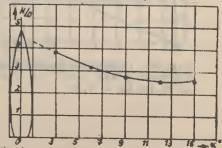
Fig. 51. Center of Pressure of the Skoda-Grenade Kodel as a Function of of at Ma = 1,4. 730
