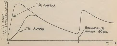
The low field strength at the start is due to the remoteness of the transmitter (about 8 km) and also to the transmitting antenna pattern. The Tur antenna rises to a higher value because it is not shadowed by the lonized jet stream until late in the flight. At the Brenuschluss point, the field atrength rises sharply because of the elimination of the jet stream.
