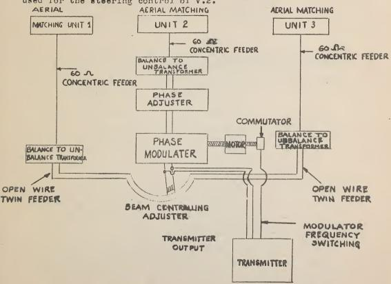
A block diagram of the ground system is shown above. The system worked on a frequency of 42mc/s. The three aerial systems were the same and each consisted of a dipole 0.44 long with a reflector of the same length spaced quarter wavelength from it. The aerials were mounted at one wavelength above the ground. The distance between the outer aerials was 20 . The transmitter used was the Lorenz 500 watt Blind approach transmitter type A.S.I.
