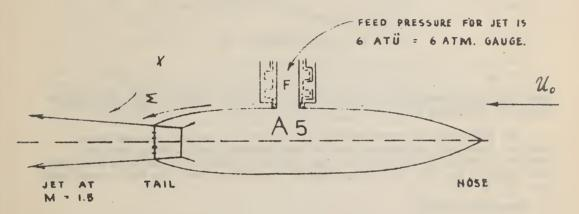
"Labyrinth Dichtung" = Maxe leak for the excess air escaping from the feed tube F was used in order to have the model freely movable around a vertical axis.
