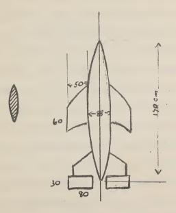
Thrust 8 ton. Stabilizing fins about seme size as the wings. Acid tank - manganese steel. Graphite blades in jet.
