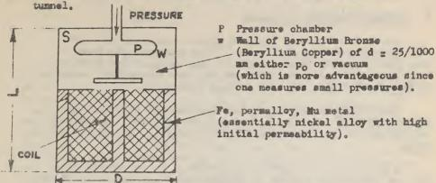
Full range for instance 5 mm Hg with an accuracy of 1% AC in the coil  $\sqrt{-\pi}$  1000 Hers. Errors given through mechanical hysteresis losses. Dimensions are of the order D  $\pi$  15 mm L  $\pi$  20 mm so they can be incorporated into the models in the wind tunnel. Space S is evacuated to a pressure at least about one hundred times smaller than the pressure one is to measure. The chamber walls on rapid evacuation must therefore be able to withstand shocks of 1 atm.
