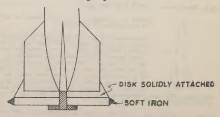
Propulsion disc rotating against the attached dime, C = centering cylinder attached to projectile. P = Pulversutter which burnt off and liberated the disc from the projectile. The burning off was achieved by a powder charge sandwiched between P and disc. (The idea of underealiber projectiles is very ald, maybe 50 years)
