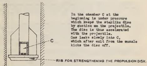
In the chamber C at the beginning is under pressure which keeps the starlike dise by suction on the projectile. The disc is thus accelerated with the projectile. Gas leaks slowly into C, which after exit from the musule kicks the disc off.
