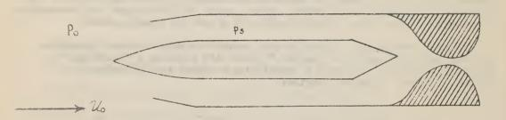
Special attention was paid the problem to achieve maximum ratio  $p_{\rm p}/p_{\rm o}$  for given  $U_{\rm D^*}$ . Oswatiatch was generally concentrating essentially on the front end intake (all the time adjusting the exhaust flow through a moveble plunger in the exit).
