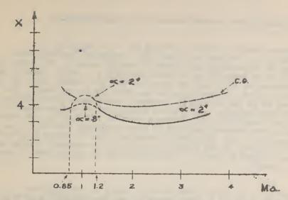
Mash manbers Ha~ I cannot be used in the wind tunnel because the hand shock wave of the model gets reflected as shock waves tither on the galls walls of the tunnel or as rerefaction waves on the interface Settless The flow and the surrounding air.
