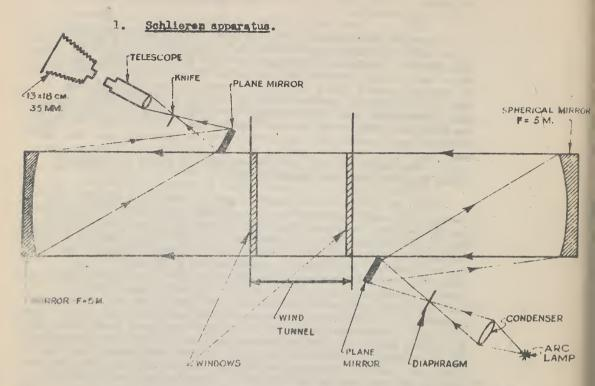
There are 2 Schlieren equipments as above, one of which is used in the tunnel. One mirror of each pair of mirrors in the tunnel spherical and the other has hyperbolic correction which is made by hand. The second equipment has two parabolic mirrors of f = 5m. The dismeter of all four mirrors is 50 cm.
