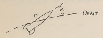
The angle of attack at the time of the propellant cut off is different for different setual orbits. The drag coefficient de pends on this angle.
