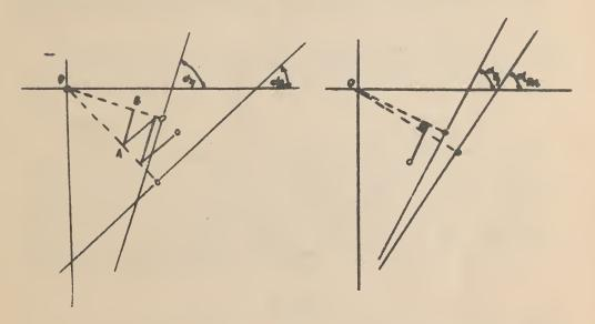
If this is made variable in relation to  $L_1$ , the locus line cuts out the sections:  $Q = R_2 R_3 - R_1 R_4 - \omega^2 \left[ L_2 L_3 - \frac{L_4}{R_4} \left( R_3 L_2 + R_2 L_3 - R_1 L_4 \right) \right]$
