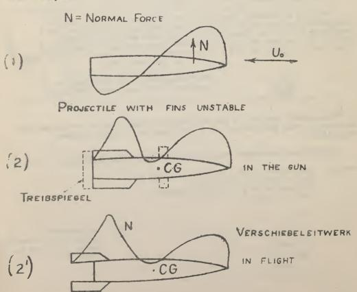
In case 3) the fine were attached to a sliding sleeve which was thrown backwards and the pressure distribution got a larger lever against CG thus etabilising the projectile.
