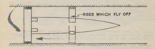
(The Fronch also had an uniorcalibor projectile which was immersal is a low melting alloy sleeve).
