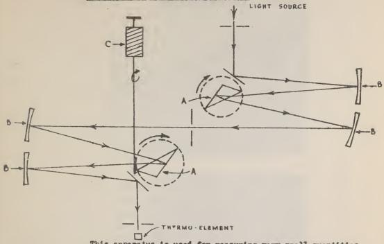
This apparatus is used for measuring very small quantities of water vapor in the air of the tunnel. Monochromatic infra-rays are passed through the tunnel and fall on a thermo-element which is connected to a galvanometer so that the absorption of the radiation in perfectly dry air can be compared with that in air containing a small quantity of water.
