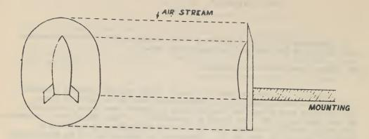
For subsenic flow the halving of the model and backing by a flat plate does not work. Models of the bisected type shown were of course used only for pressure measurements and not for drag, lift and moments.
