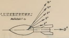
Fig. 36. Vectors Showing Magnitude, Direction and Centers of Pressure for the Aerodynamic Forces Acting on the Fin-Grenade Model at Ma = 1,8.
