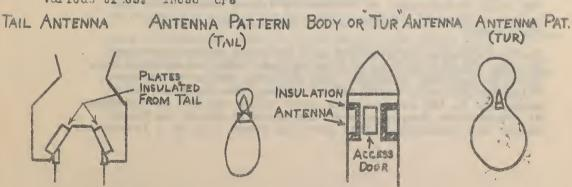
The tail antennas consist either a pair or dipoles red an op osite phase
