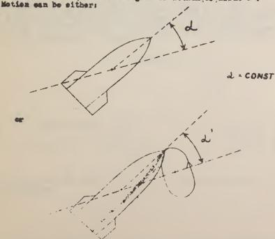
laterference of the boundary Doyer with the fine is disturbing especially when there is a finite angle of attack as the sketch shows.
