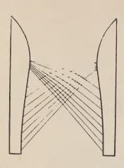
Fig. 7 Supersonic Nozzle for Ma = 1,57 Supersonic Nozzle for Ma = 1,88 (540 m/sec.)
