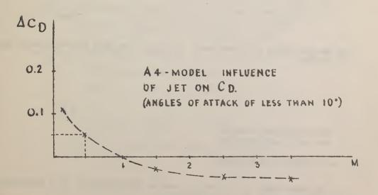
The astmal paths of the  $A_{\lambda}$  were not actually analyzed for the influence of the jet on  $C_D$  of the whole missile. Lift coefficient with the jet were not determined.
