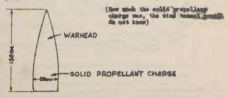
Empoles Caliber 28 cm, L = 5,36 b. Musale velocity 1000 m/acc. Maximum after the additional propulsion is most known. Dispersion is they bad, because reaket propulsion is applied in various directions depending on the inclination of the projection at the memory of ignification.
