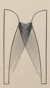
Fig. 9 Supersonic Nozzle for Na = 2.5 Supersonic Nozzle for Ma 3,3 (850 m/sec.)
