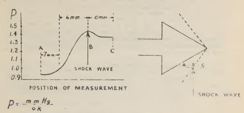
Measurements were made at various point parallel to the axis of the model along a line crossing the shock wave as shown. There is a break in the pressure curve at this point. The decrease in pressure beyond B was not expected; it may be that some molecular process (rotation, vibra ion?) proceeds too slowly to absorb the energy of the shock wave without having the pressure rise above its final value.
