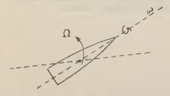
If  $\omega \sim \Omega$  the tumbling occurs. Since  $\Omega \sim 1$  to 10 Hz. Therefore the undercaliber projectiles were given inclined fins to produce the necessary large  $\omega > \Omega$  right away.
