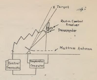
The radar was used solely for tracking the target and actuating a transponder aboard the missile. A separate receiving mattress would then track the rocket by the transponded signal. The bearing angles of the two entennes would then be compared and an appropriate control signal sent to the rocket to bring it back into the beam. It was developed for line-of-sight operation but some thought was given to collision course speration.
