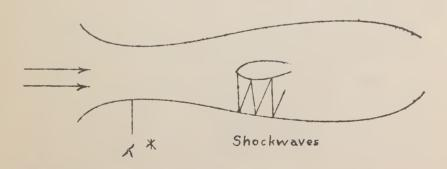
Near Ma = 1 the pressure centers come dangerously near the CG. To make sure that nothing would happen at Ma = 1 with the A, similar bodies were dropped from planes from 8000 meters height and observed in their transition through Ma = 1 at about 1000 meters altitude. A, flow up to Ma = 5 at a soint which solucided closely with "Brennschluß" = propellant out-off.
