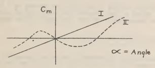
Only  $\mathbf{c}_n$ 's of the type I could be managed, both for the  $\mathbf{c}_n$  of the main body and the rudders.
