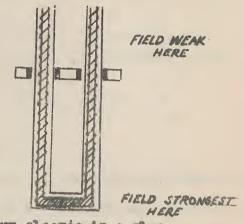
consisted of a shorted turn of aluminum sleeves in a glass float. 1% accuracy on alcohol. Wanted 1%, but could not get this with these continuous instruments so changed to two new instruments giving signals at 10 levels.
