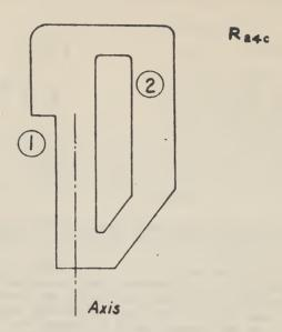
The pressure peak at (1) is presumably counter balanced (in its effect on the torque around the axis) by a new pressure peak at (2).
